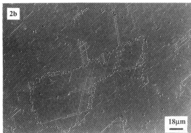
Figure 2. Crystalline arrays of monodisperse, polystyrene microspheres, diameter = 1.78\text{-}\mu\text{m} (view angle 90^\circ ). Areas of perfect dense packings are separated by crystal fault lines. (a) Scanning electron micrograph; (b) optical micrograph.
